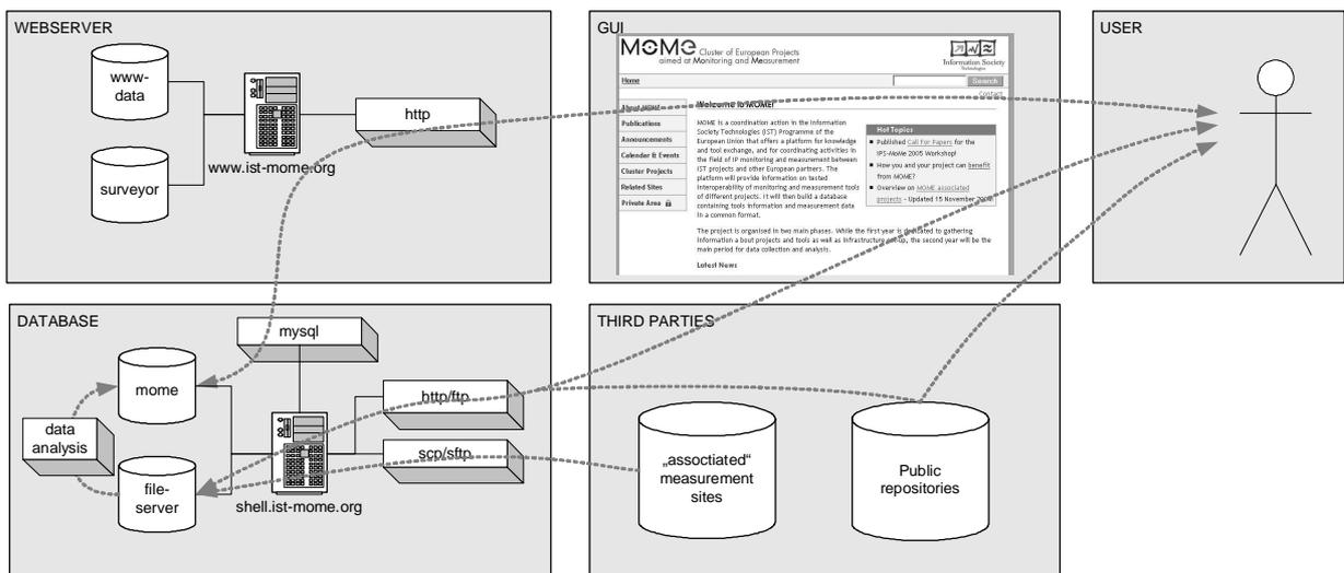
Figure 2. Deployment of the MOME meta-repository
